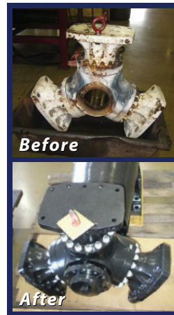
Fesco Wind Turbine Gear Box Reconditioning
