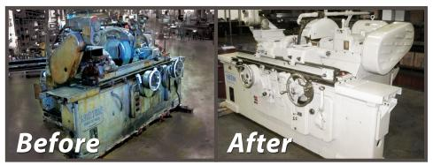
Norton Grinder Machine Rebuild
