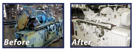
Norton Grinder Machine Rebuild
